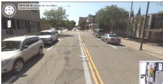
Match 700 Block of Third 11' wide sidewalk both sides (18) 7'x23' parallel parking stalls, (9) per side vs e(14) angled stalls existing (2) 12'-6" wide drive lanes
